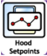
The Hood Setpoints menu button provides access to adjust setpoint parameters used by the NB-FHC to perform fume hood control. Within this menu, operators can monitor and modify the current Face Velocity setpoint, directly affecting PID Control performance of the Exhaust Damper Output. Any user (logged in or not) has the ability to monitor the Face Velocity Setpoint.
